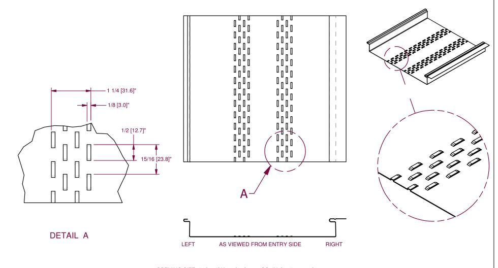
OPENING SIZE .50 [12.7] X .12 [3.0] = .06 SQ. IN. [38.7 sq. mm] OPENINGS PER 12 INCH LENGTH [304.8 mm] = 51.25 NET FREE AREA / 12 INCH = .06 SQ IN X 51.25 = 3.08 SQ IN. [net free area / 304.8 mm = 38.7 sq. mm X 51.25 = 1983 sq. mm]
